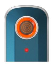
Blinking Green: Firefly 2 is heating. Solid Green: Firefly 2 is ready to use.
